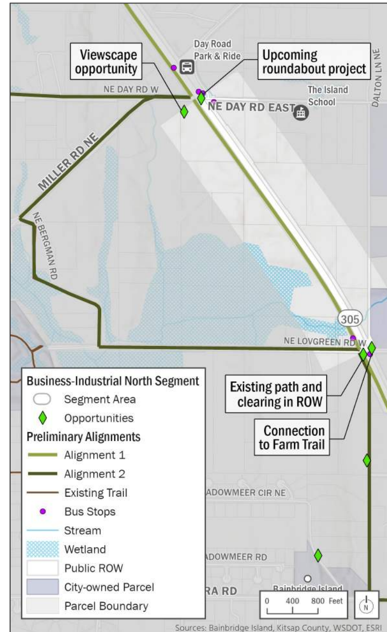
Figure 16. Business-Industrial North Segment: Alignment Alternatives
