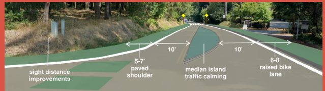
East facing view of Design Alternative D on Wyatt Way NW at the intersection of Wyatt and Finch Road NE.
