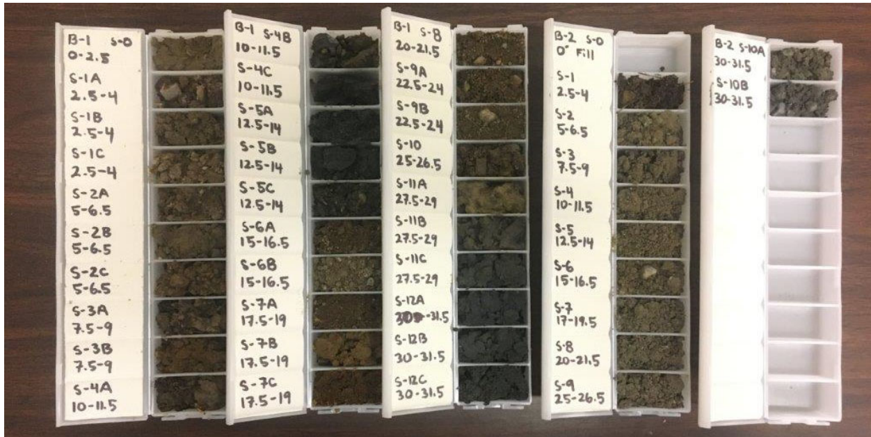
Photo 1. Reference sample trays created from samples for exploration borings B-1 and B-2.
