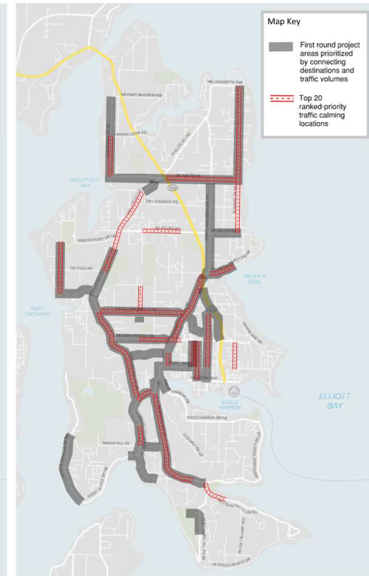
Step 3. Overlap top 20 traffic calming locations as determined by traffic calming evaluation process.
