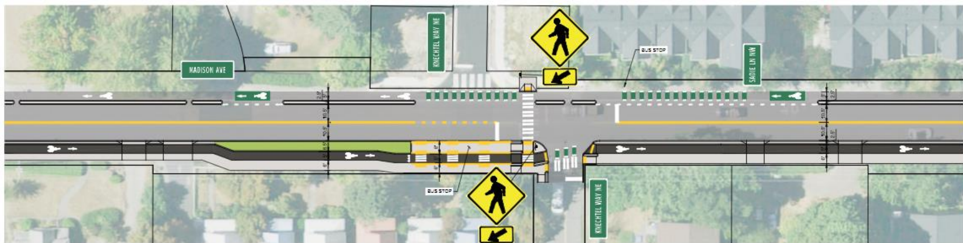
CENTRAL SEGMENT (WYATT WAY TO HIGH SCHOOL ROAD) OPTION B: NORTHBOUND SIDEWALK LEVEL BIKE LANE, SOUTHBOUND STREET LEVEL BIKE LANE
