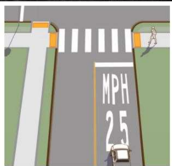
SLOW or Speed Limit Pavement Legends
