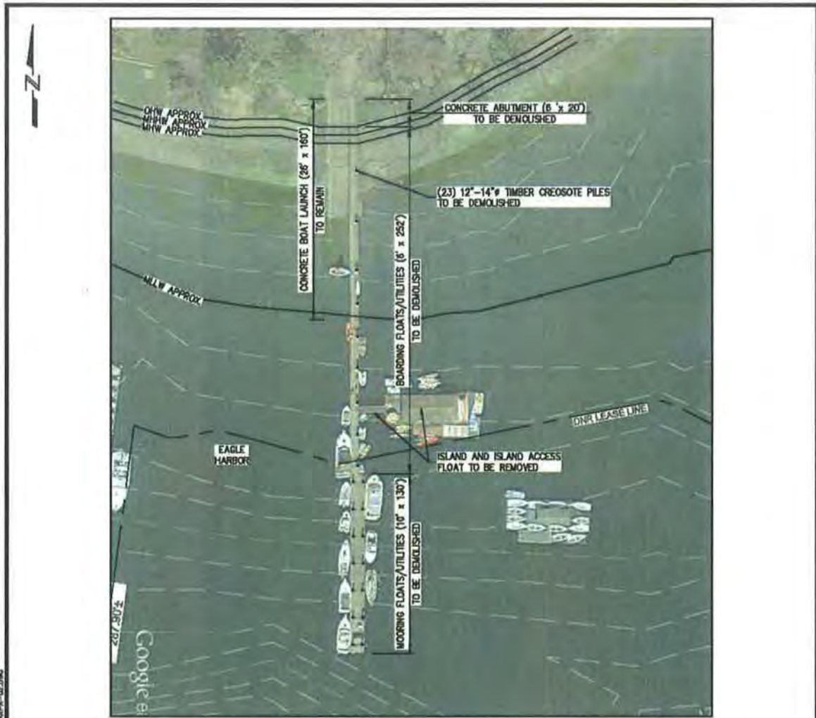
EXISTING CONDITIONS AND DEMOLITION PLAN 0 25 50 75 150 APPROXIMATE SCALE
